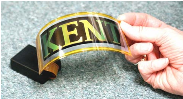
FIGURE 1. Bistable flexible cholesteric display showing flexibility. The display in the photograph is made of two 50 \mu m substrates.
