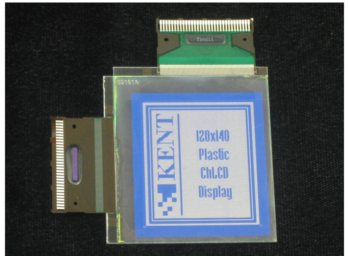
Figure 2: Flexible display made with 125µm PET substrates and ITO as conductor. The drivers are off-the-shelf LCD drivers.
