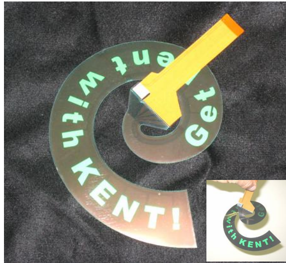
Fig. 2 A “spiral” display made from patterned ITO on 2mil PET. Inset: the display takes a helical shape when hanging.
