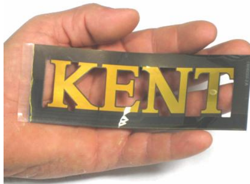
Fig. 1 Laser edge sealed ITO-based display. Inactive portions of the display were laser edge sealed and removed.
