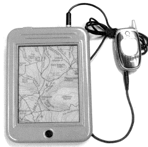
Figure 5. Reflex™ display including a solar cell behind the display. The solar cell not only powers the display but also generates enough additional energy to charge other devices.
