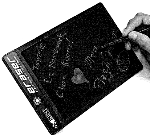
Figure 3. Flexible Reflex™ writing tablet display only requires power when the written notes are no longer needed and are erased.
