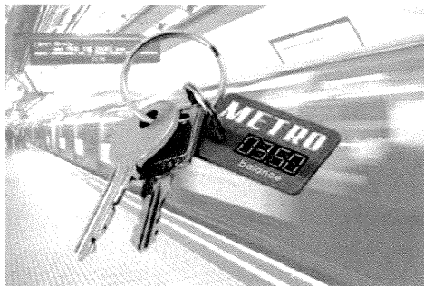
Figure 10. Flexible Reflex™ smart card display allows versatile card design. Since Reflex™ displays only require power upon changing the image the battery can be located in the card or on an external card fixture, only powering the display when swiped.
