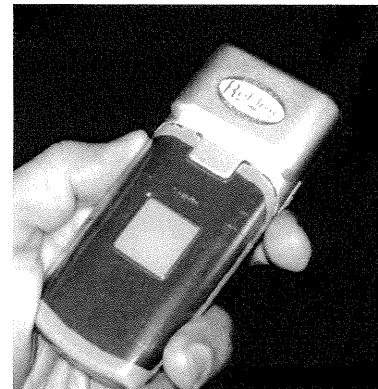
Figure 7. Flexible Reflex™ electronic skin. Consumers can have ultra personalized color without draining precious battery life.
