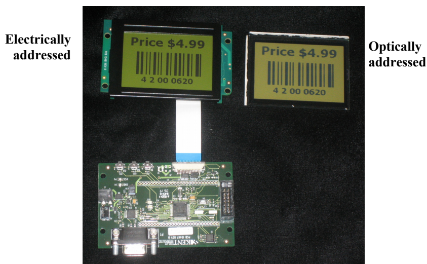
Figure 9: A conventional display (left) with attached bulky and costly electronics compared with an optically addressed display (right) with the same image without the added electronics.
