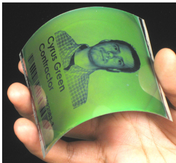
Figure 1: A flexible optically addressed photochiral display. The display shown here is flexed and based on flexible ChLCD technology.
