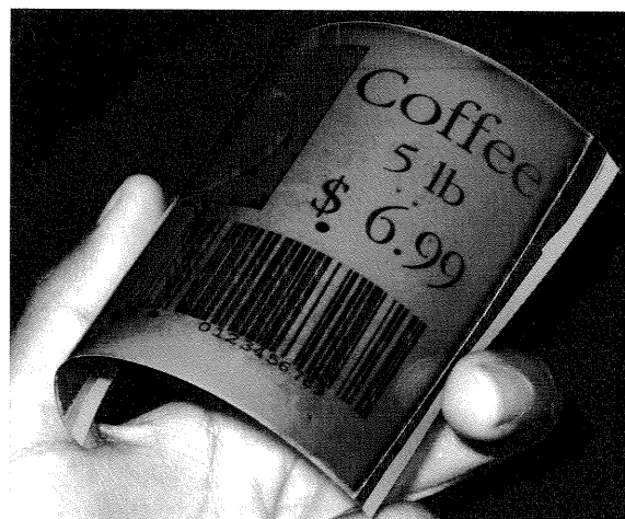
Figure 1. An optically addressed flexible photochiral display
